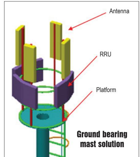
street lighting, billboards and security cameras can be installed on the exterior. This design is built to withstand wind speeds of 180 kmph. Moreover, the electrical and grounding system complies with various local standards.
